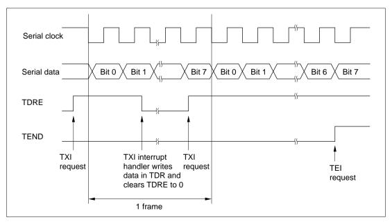
Figure 12.14 Example of SCI Transmit Operation
