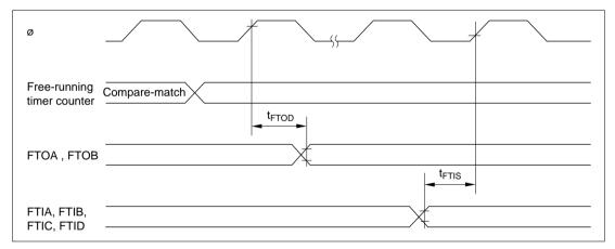
Figure 23.13 Free-Running Timer Input/Output Timing
