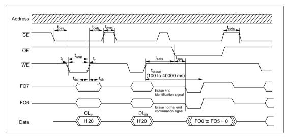
Figure 21.21 Auto-Erase Mode Timing Waveforms
