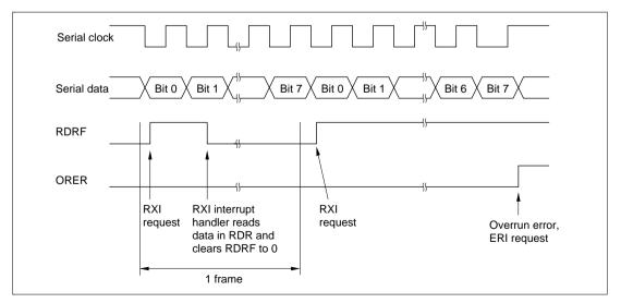
Figure 12.16 Example of SCI Receive Operation
