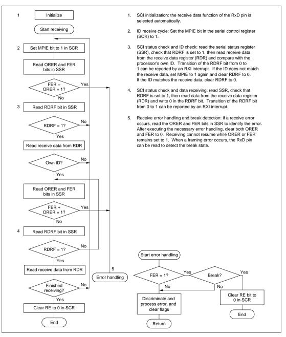
Figure 12.10 Sample Flowchart for Receiving Multiprocessor Serial Data
