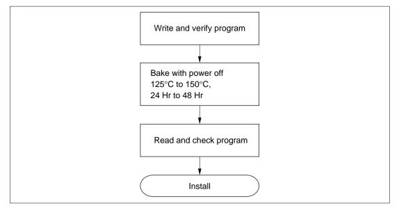
Figure 18.7 Recommended Screening Procedure
