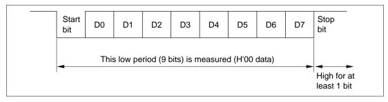
Figure 21.8 Measurement of Low Period in Data Transmitted from Host
