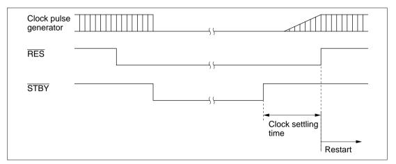
Figure 22.2 Hardware Standby Mode Timing
