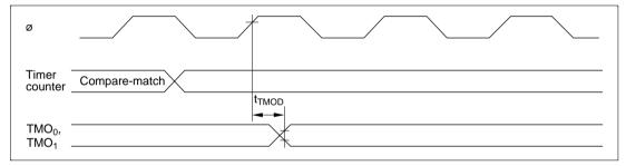
Figure 23.15 8-Bit Timer Output Timing
