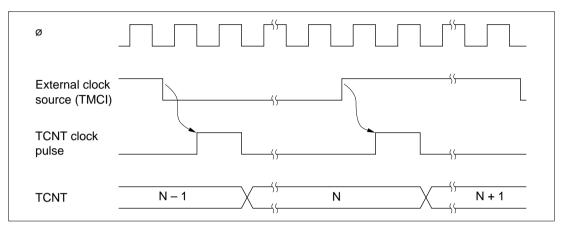
Figure 9.3 Increment Timing for External Clock Input
