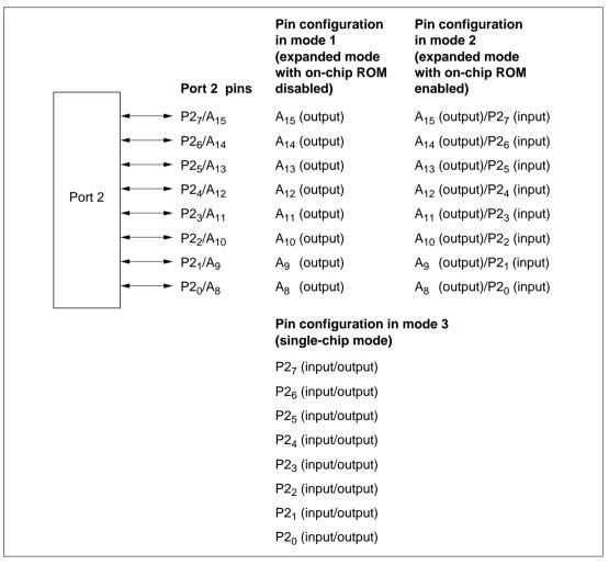
Figure 7.5 Port 2 Pin Configuration
