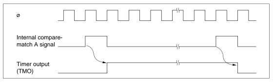
Figure 9.5 Timing of Timer Output
