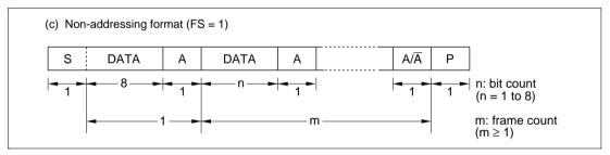
Figure 13.4 I<sup>2</sup>C Bus Data Format (Non-Acknowledge Format)
