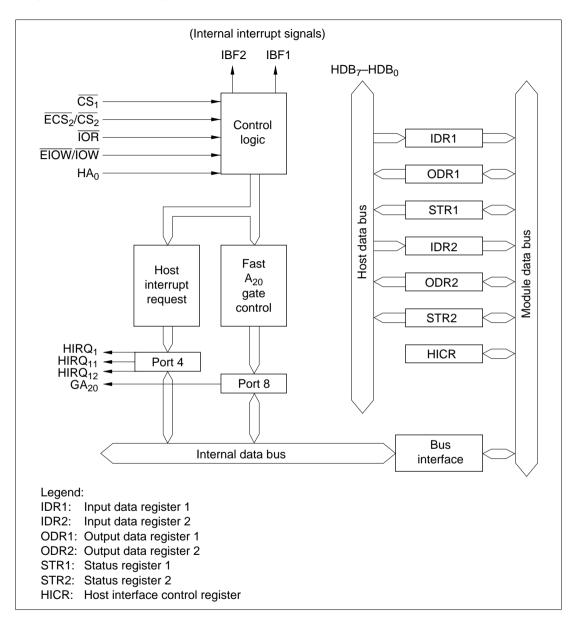
Figure 14.1 is a block diagram of the host interface.
