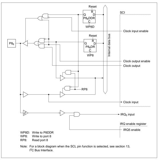
Figure C.8 (f) Port 8 Block Diagram (Pin P8<sub>6</sub>)
