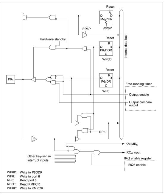
Figure C.6 (c) Port 6 Block Diagram (Pin P6<sub>6</sub>)
