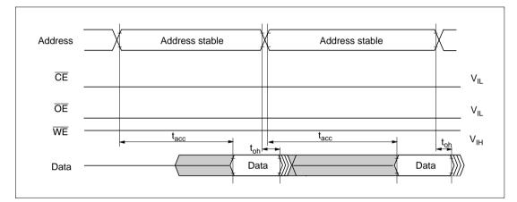
Figure 21.18 Timing Waveforms for  $\overline{CE}$  and  $\overline{OE}$  Enable State Read
