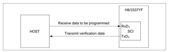
Figure 20.3 Boot-Mode System Configuration
