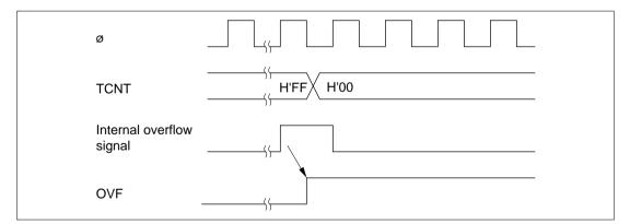
Figure 11.5 Setting the OVF Bit
