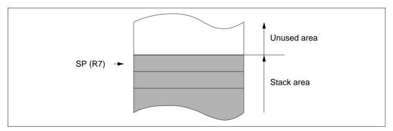
Figure 2.2 Stack Pointer
