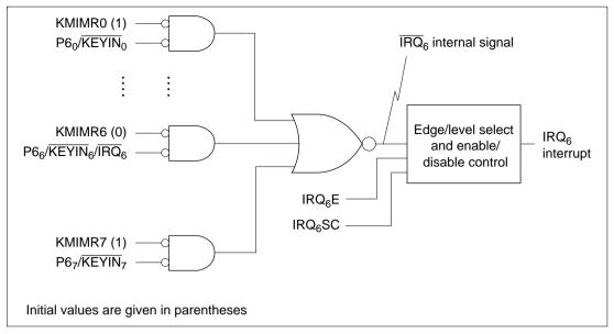
Figure 4.3 KMIMR and IRQ<sub>6</sub> Interrupt
