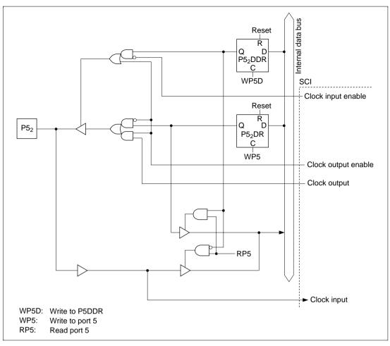
Figure C.5 (c) Port 5 Block Diagram (Pin P5<sub>2</sub>)
