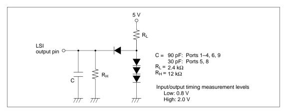
Figure 23.3 Output Load Circuit
