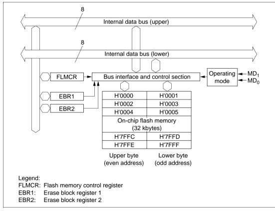
Figure 19.1 Flash Memory Block Diagram
