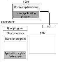
On-board update routine transfer The transfer program in the flash memory is executed, and the on-board update routine is transferred to RAM.
