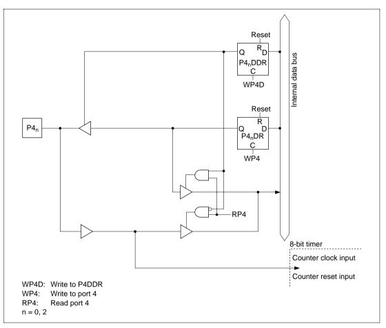
Figure C.4 (a) Port 4 Block Diagram (Pins P4<sub>0</sub>, P4<sub>2</sub>)
