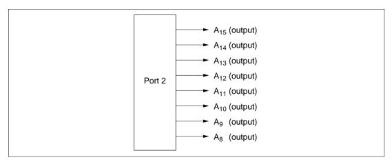
Figure 7.6 Pin Functions in Mode 1 (Port 2)
