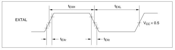
Figure 6.6 External Clock Input Timing
