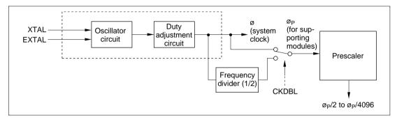
Figure 6.1 Block Diagram of Clock Pulse Generator
