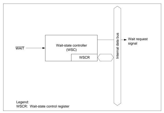
Figure 5.1 Block Diagram of Wait-State Controller
