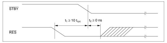
(2) When the RAME bit in SYSCR is cleared to 0 or when it is not necessary to retain RAM contents, RES does not have to be driven low as in (1).
