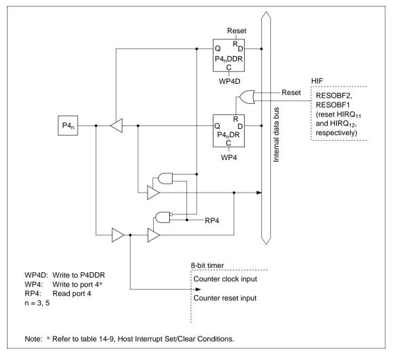
Figure C.4 (c) Port 4 Block Diagram (Pins P4<sub>3</sub>, P4<sub>5</sub>)
