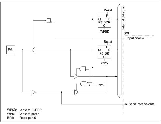
Figure C.5 (b) Port 5 Block Diagram (Pin P5<sub>1</sub>)
