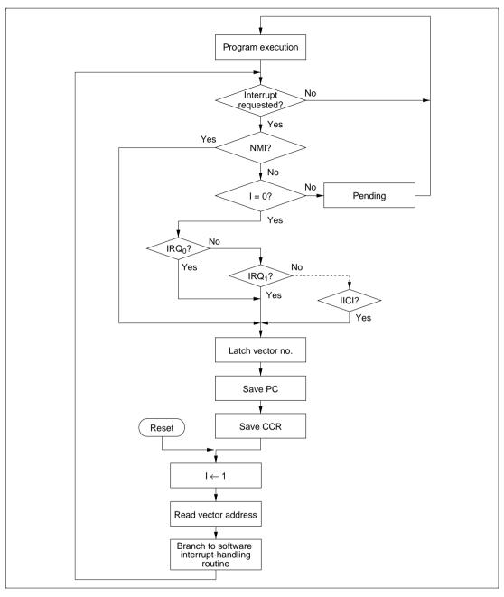
Figure 4.5 Hardware Interrupt-Handling Sequence
