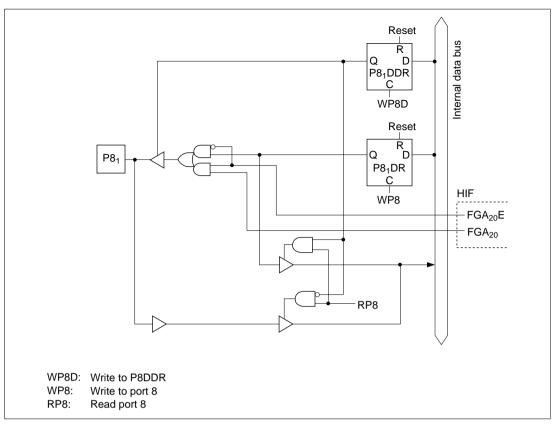
Figure C.8 (b) Port 8 Block Diagram (Pin P8<sub>1</sub>)
