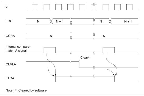
Figure 8.6 Timing of Output Compare A
