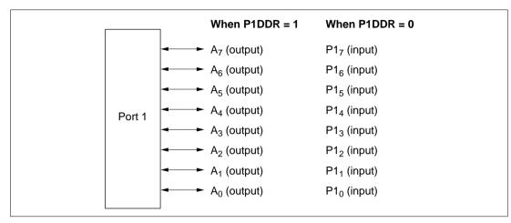
Figure 7.3 Pin Functions in Mode 2 (Port 1)
