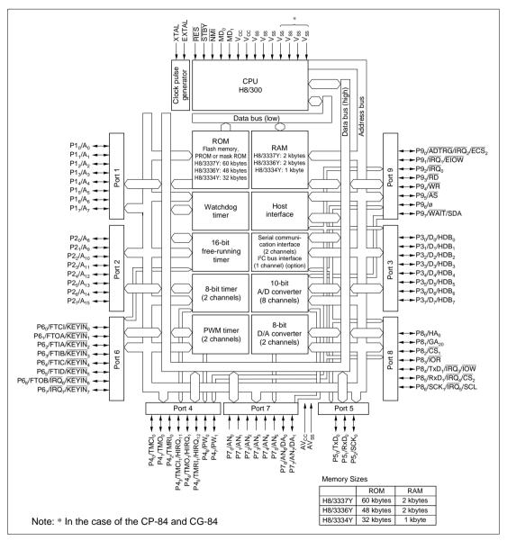
Figure 1.1 (a) Block Diagram for H8/3337 Series
