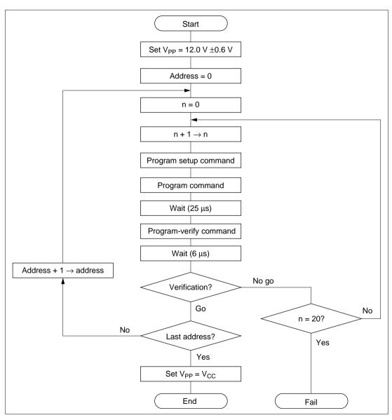
Figure 19.15 High-Speed, High-Reliability Programming
