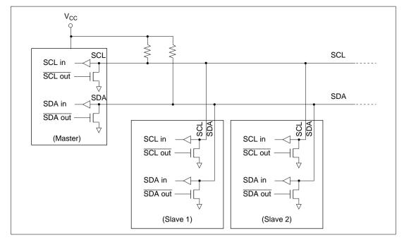
Figure 13.1 I<sup>2</sup>C Bus Interface Connections (Example) (H8/3337 Series Chip as Master)
