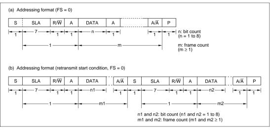
Figure 13.3 I<sup>2</sup>C Bus Data Formats (Acknowledge Formats)
