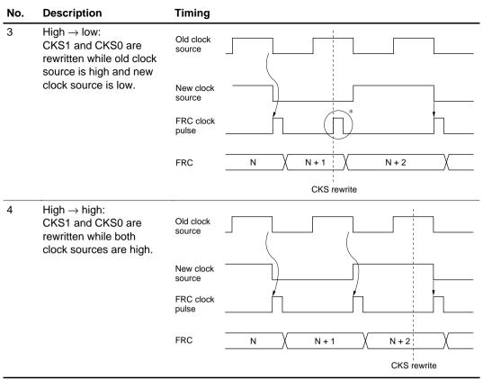
Note: \* The switching of clock sources is regarded as a falling edge that increments FRC.
