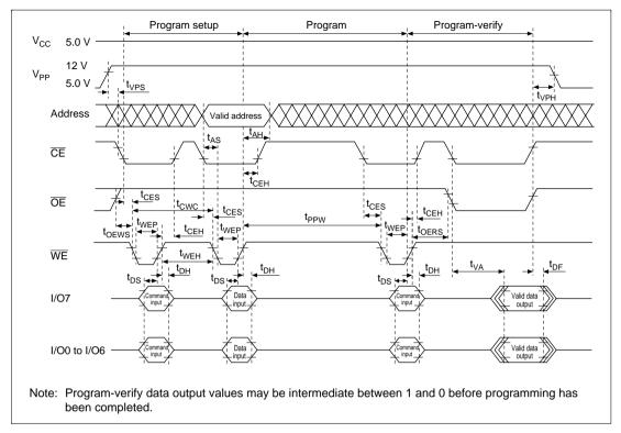
Figure 20.18 High-Speed, High-Reliability Programming Timing
