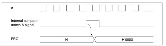
Figure 8.7 Clearing of FRC by Compare-Match A
