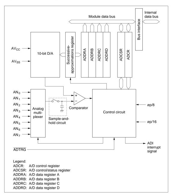
Figure 15.1 shows a block diagram of the A/D converter.
