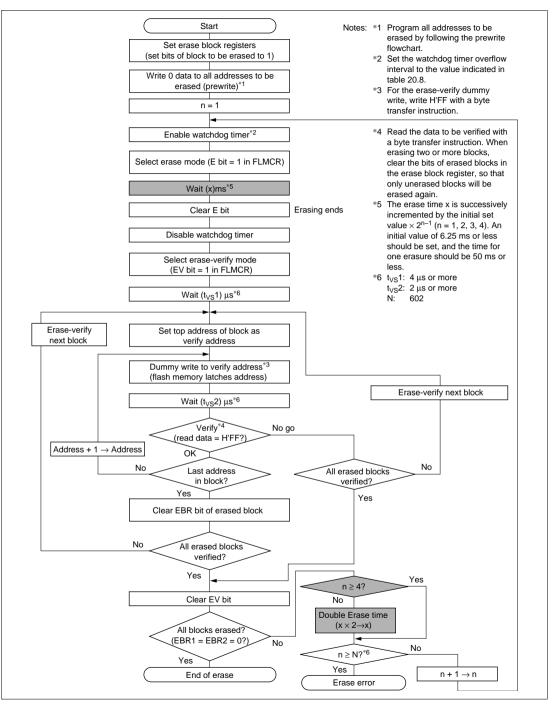
Figure 20.11 Multiple-Block Erase Flowchart
