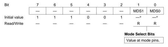
Note: \* Determined by inputs at pins MD<sub>1</sub> and MD<sub>0</sub>.
