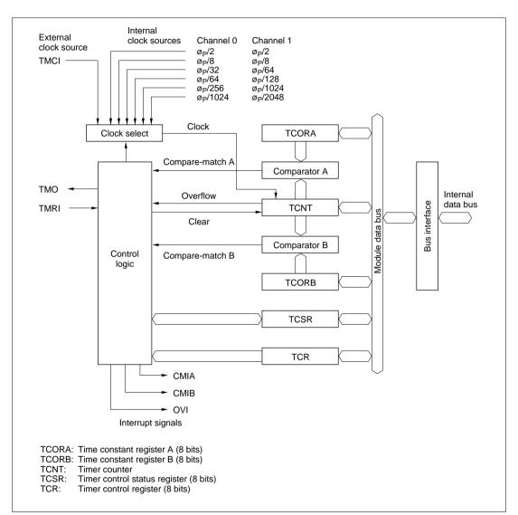
Figure 9.1 shows a block diagram of one channel in the 8-bit timer module.
