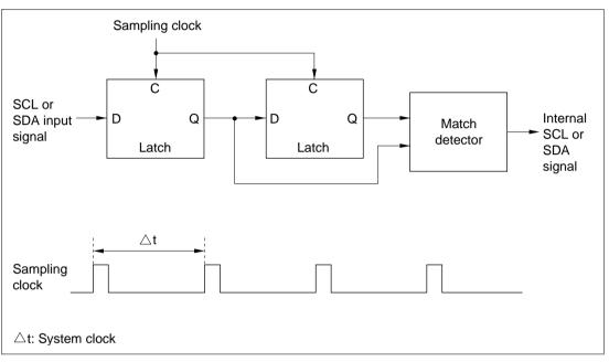
Figure 13.11 Block Diagram of Noise Canceler
