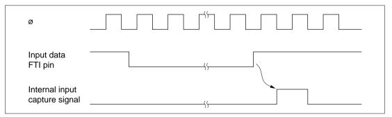
Figure 8.8 Input Capture Timing (Usual Case)
