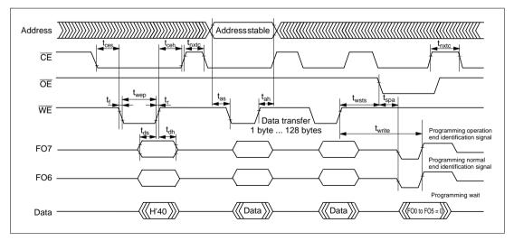
Figure 21.20 Auto-Program Mode Timing Waveforms
