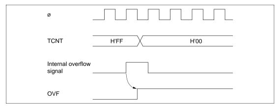
Figure 9.8 Setting of Overflow Flag (OVF)
