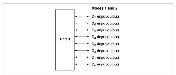
Figure 7.10 Pin Functions in Modes 1 and 2 (Port 3)
