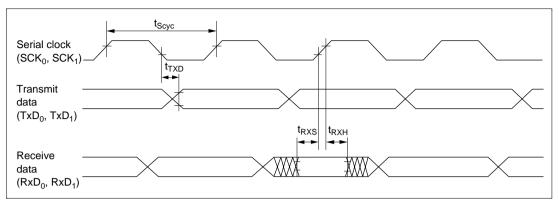
Figure 23.19 SCI Input/Output Timing (Synchronous Mode)
