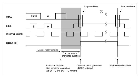
Figure 13.21 Precautions when Reading Master Receive Data
