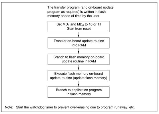
Figure 21.11 User Programming Mode Operation (Example)
