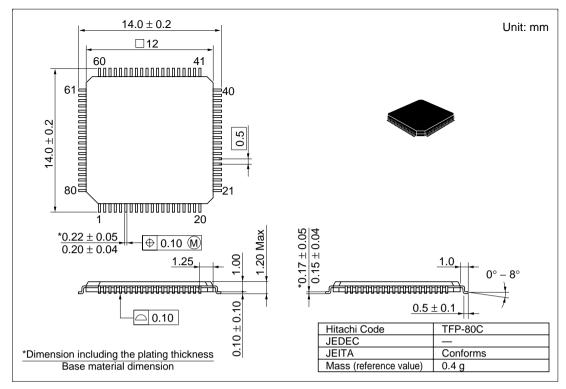
Figure H.2 Package Dimensions (TFP-80C)
