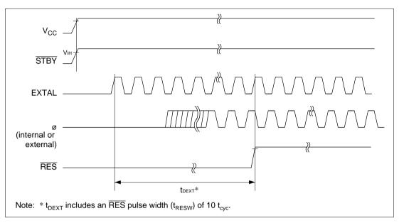
Figure 23.25 External clock output delay Timing
