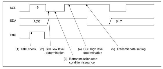
Figure 13.17 Timing Chart for Retransmission Start Condition Issuance
