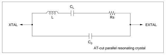
Figure 6.3 Equivalent Circuit of External Crystal
