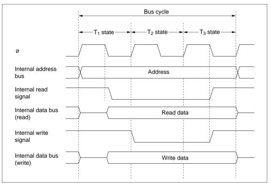
Figure 2.15 On-Chip Supporting Module Access Cycle
