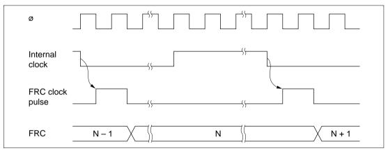
Figure 8.4 Increment Timing for Internal Clock Source
