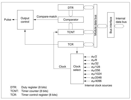
Figure 10.1 Block Diagram of PWM Timer (One Channel)
