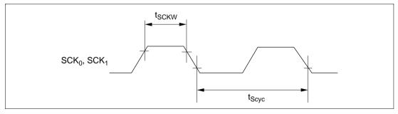
Figure 23.20 SCI Input Clock Timing
