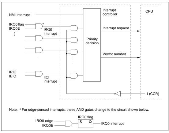
Figure 4.4 Block Diagram of Interrupt Controller
