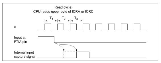
Figure 8.11 Input Capture Timing (1-State Delay, Buffer Mode)
