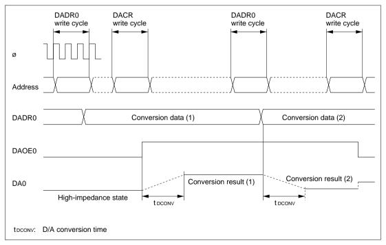
Figure 16.2 D/A Conversion (Example)
