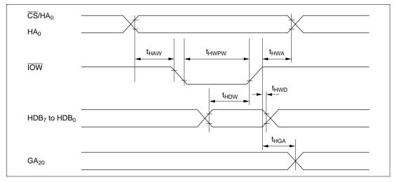
Figure 23.23 Host Interface Write Timing
