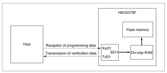
Figure 21.6 Boot-Mode System Configuration
