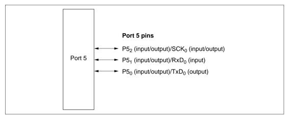
Figure 7.13 Port 5 Pin Configuration
