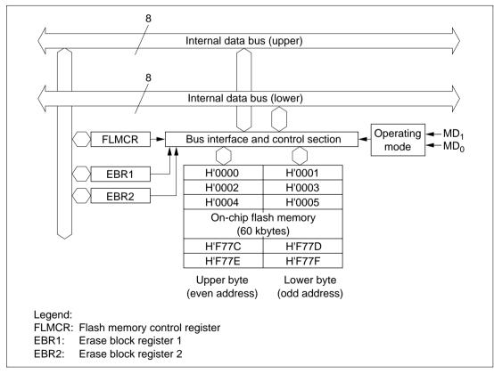
Figure 20.1 Flash Memory Block Diagram
