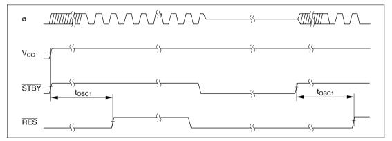
Figure 23.11 Clock Settling Timing
