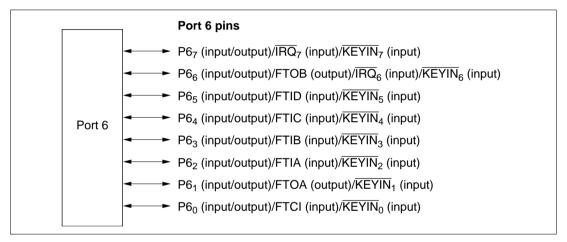
Figure 7.14 Port 6 Pin Configuration
