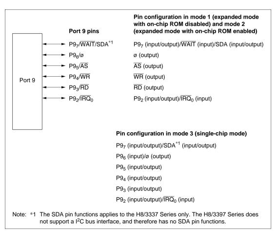
Pin  $9_7$  can drive a bus buffer. For details, see section 13, I<sup>2</sup>C Bus Interface.
