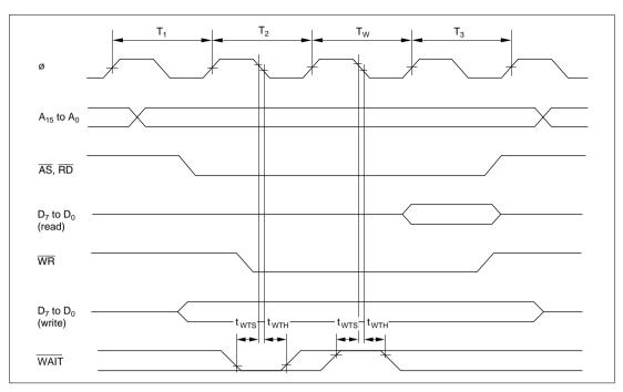
Figure 23.8 Basic Bus Cycle (with 1 Wait State) in Expanded Modes (Modes 1 and 2)
