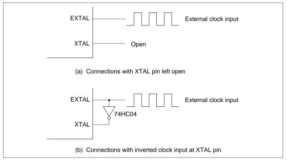
Figure 6.5 External Clock Input (Example)
