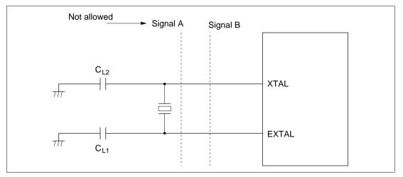
Figure 6.4 Board Design around External Crystal
