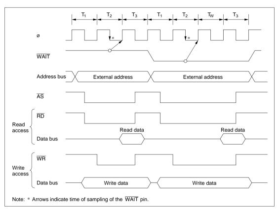
Figure 5.4 shows the timing when the wait count is 1.
