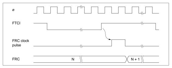
Figure 8.5 Increment Timing for External Clock Source
