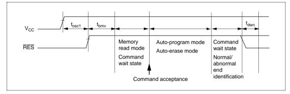
Figure 21.23 Oscillation Settling Time, Boot Program Transfer Time, and Power-Down Sequence
