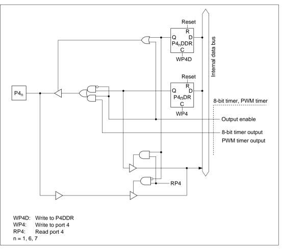
Figure C.4 (b) Port 4 Block Diagram (Pins P4<sub>1</sub>, P4<sub>6</sub>, P4<sub>7</sub>)
