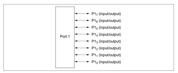
Figure 7.4 Pin Functions in Mode 3 (Port 1)
