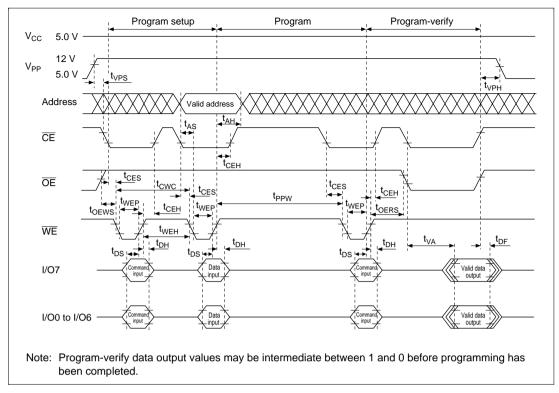
Figure 19.18 High-Speed, High-Reliability Programming Timing
