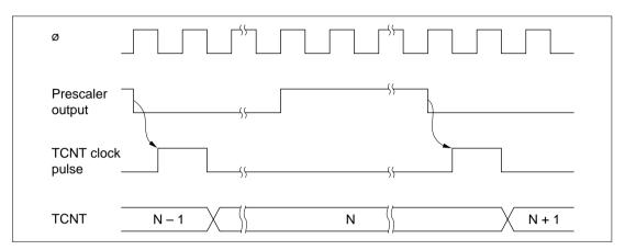
Figure 10.2 TCNT Increment Timing
