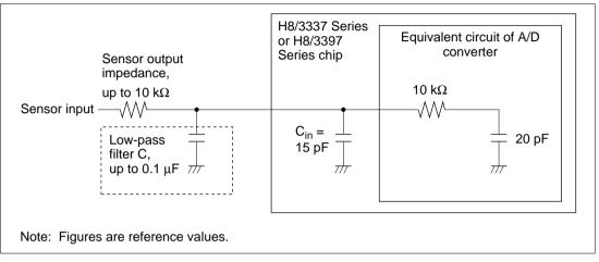
Figure 15.10 Example of Analog Input Circuit
