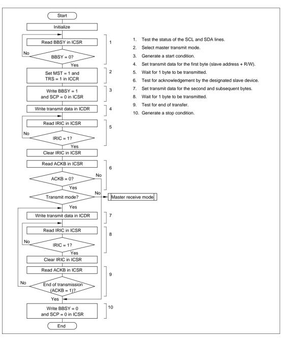
Figure 13.12 Flowchart for Master Transmit Mode (Example)
