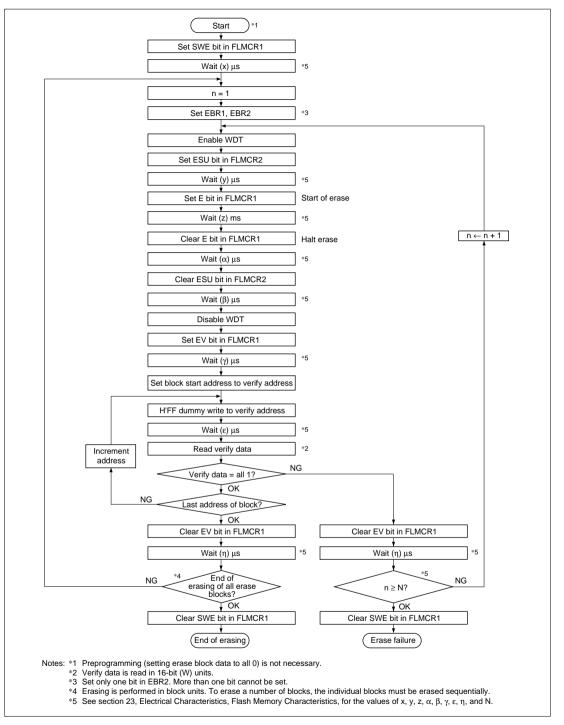
Figure 21.13 Erase/Erase-Verify Flowchart (Single-Block Erase)
