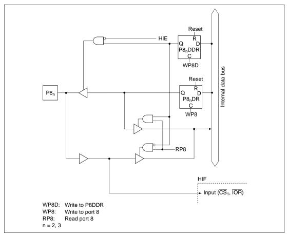
Figure C.8 (c) Port 8 Block Diagram (Pins P8<sub>2</sub>, P8<sub>3</sub>)
