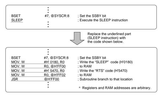
Note: When a SLEEP instruction is executed in ROM, the current responsible for this bug also flows when a sleep mode transition is made. Therefore, to further reduce current dissipation in sleep mode, also, software should be modified so that the SLEEP instruction is executed in RAM when making a sleep mode transition.
