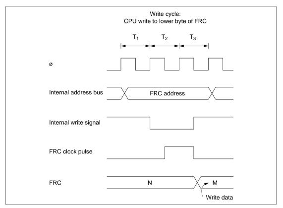
Figure 8.17 FRC Write-Increment Contention
