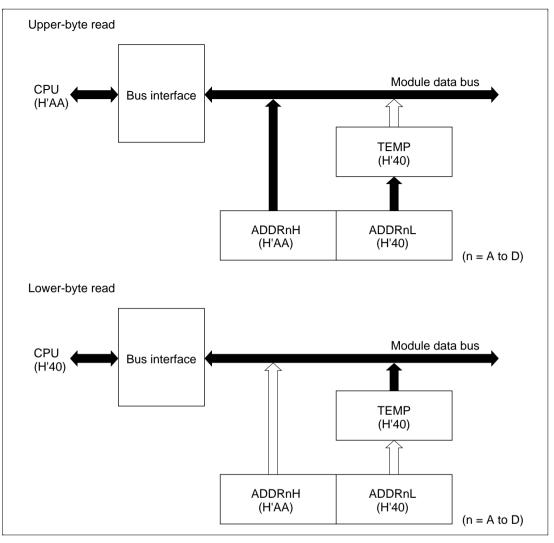
Figure 15.2 A/D Data Register Access Operation (Reading H'AA40)
