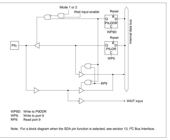
Figure C.9 (f) Port 9 Block Diagram (Pin P97)
