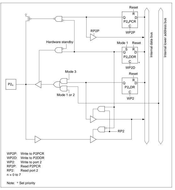
Figure C.2 Port 2 Block Diagram
