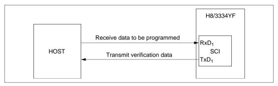
Figure 19.3 Boot-Mode System Configuration
