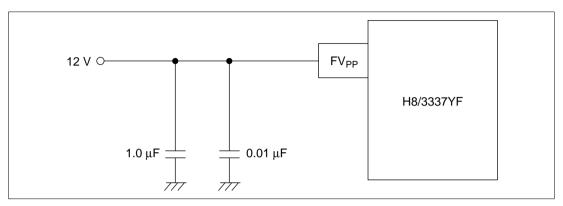
Figure 20.21 V<sub>PP</sub> Power Supply Circuit Design (Example)
