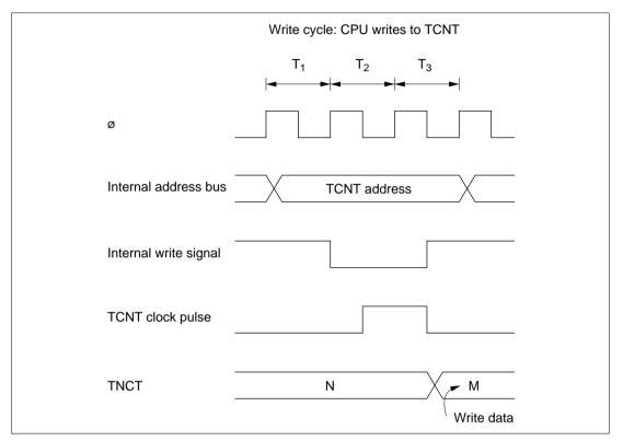
Figure 9.11 TCNT Write-Increment Contention
