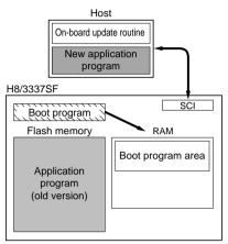
4. Writing new application program The on-board update routine in the host to RAM is transferred to RAM by SCI communication and executed, and the new application program in the host is written into the flash memory.
