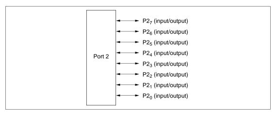
Figure 7.8 Pin Functions in Mode 3 (Port 2)
