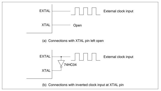
Figure 6.11 External Clock Input (Example)
