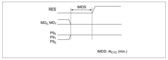
Figure 21.10 Programming Mode Timing
