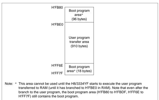
Note also that 16 bytes (H'FB80 to H'FB8F) of this area cannot be used if an interrupt handling routine is executed within the boot program. For details see section 19.4.9, Interrupt Handling during Flash Memory Programming and Erasing.
