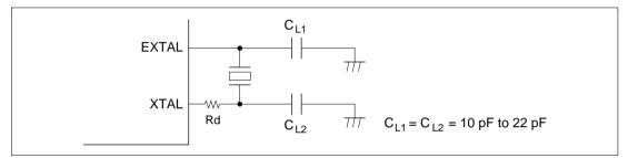
Figure 6.2 Connection of Crystal Oscillator (Example)
