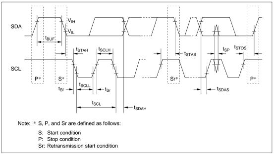
Figure 23.24 I<sup>2</sup>C Interface Input/Output Timing
