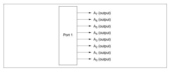
Figure 7.2 Pin Functions in Mode 1 (Port 1)
