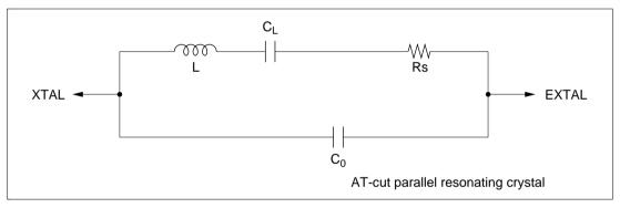
Figure 6.9 Equivalent Circuit of External Crystal
