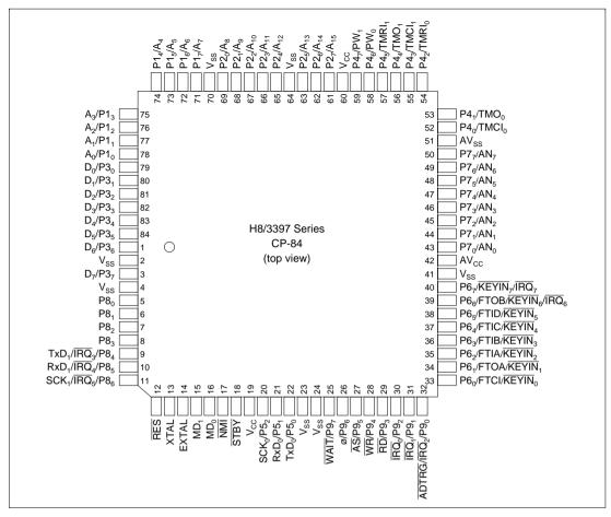
Figure 1.3 (b) Pin Arrangement for H8/3397 Series (CP-84, Top View)
