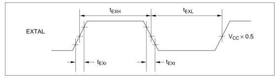
Figure 6.12 External Clock Input Timing
