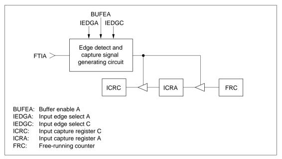
Figure 8.2 Input Capture Buffering (Example)
