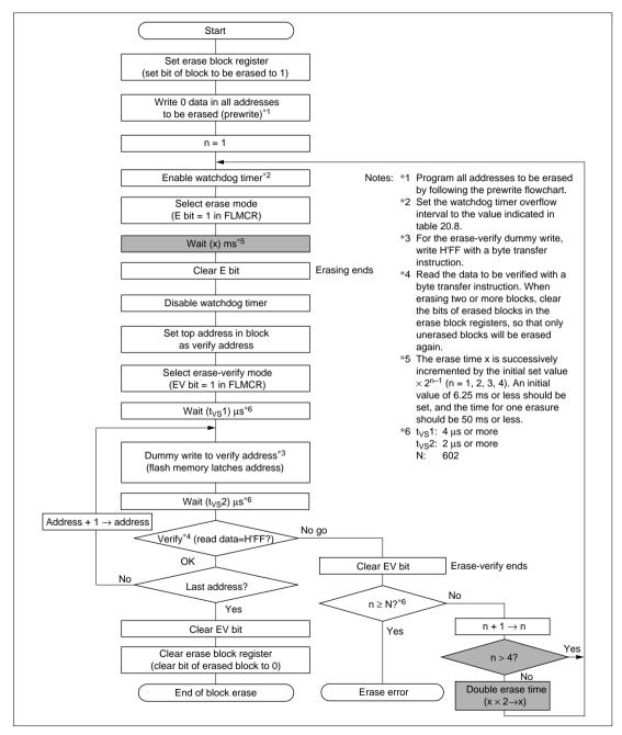
Figure 20.9 Erasing Flowchart
