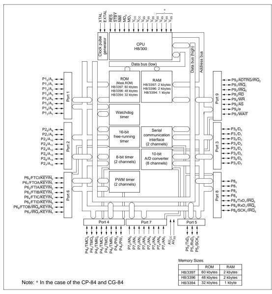
Figure 1.1 (b) Block Diagram for H8/3397 Series
