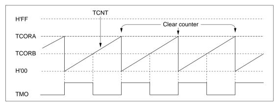
Figure 9.9 Example of Pulse Output
