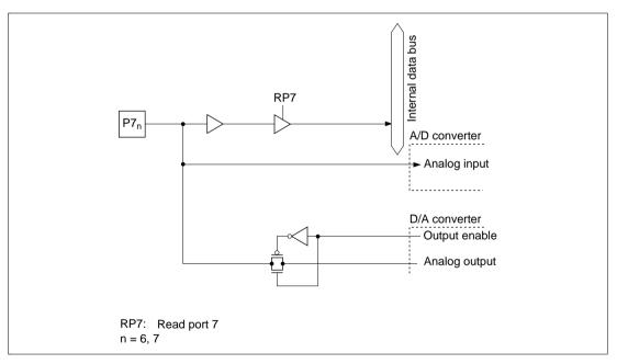
Figure C.7 (b) Port 7 Block Diagram (Pins P7<sub>6</sub> and P7<sub>7</sub>)
