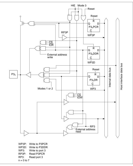
Figure C.3 Port 3 Block Diagram
