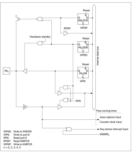
Figure C.6 (a) Port 6 Block Diagram (Pins P6<sub>0</sub>, P6<sub>2</sub>, P6<sub>3</sub>, P6<sub>4</sub>, P6<sub>5</sub>)
