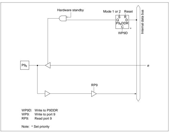
Figure C.9 (e) Port 9 Block Diagram (Pin P9<sub>6</sub>)
