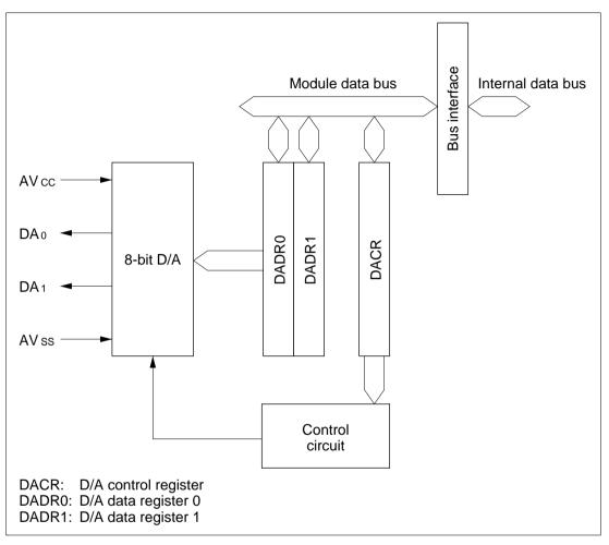
Figure 16.1 D/A Converter Block Diagram
