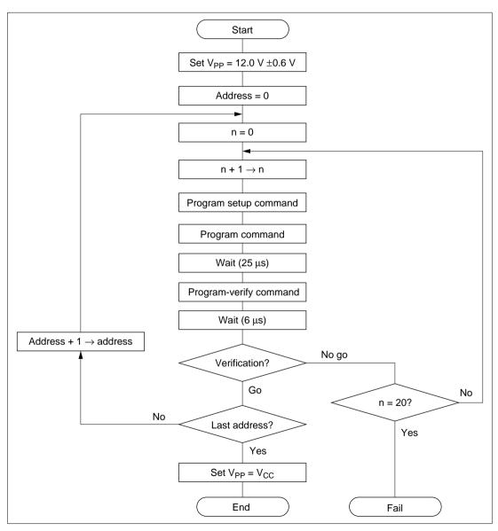
Figure 20.15 High-Speed, High-Reliability Programming
