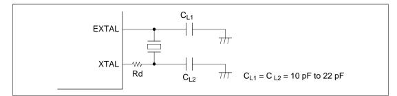
Figure 6.8 Connection of Crystal Oscillator (Example)
