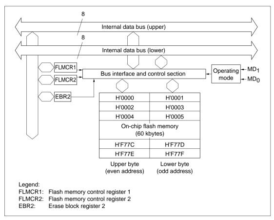
Figure 21.1 Flash Memory Block Diagram
