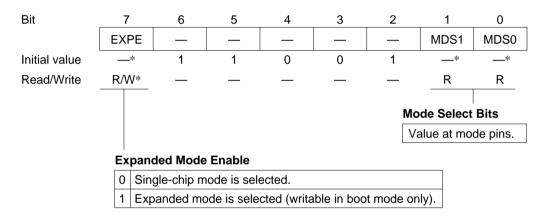
Note: \* Determined by inputs at pins  $MD_1$  and  $MD_0$ .
