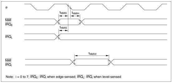
Figure 23.10 Interrupt Input Timing
