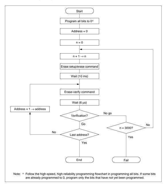
Figure 19.16 High-Speed, High-Reliability Erasing
