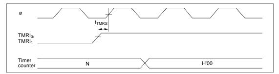
Figure 23.17 8-Bit Timer Reset Input Timing
