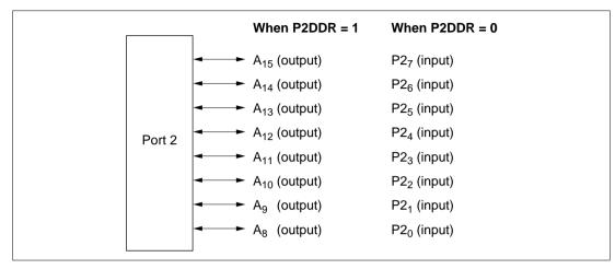
Figure 7.7 Pin Functions in Mode 2 (Port 2)
