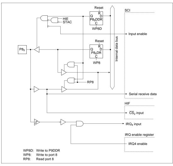
Figure C.8 (e) Port 8 Block Diagram (Pin P85)
