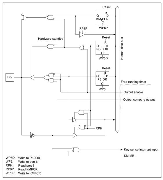
Figure C.6 (b) Port 6 Block Diagram (Pin P6<sub>1</sub>)
