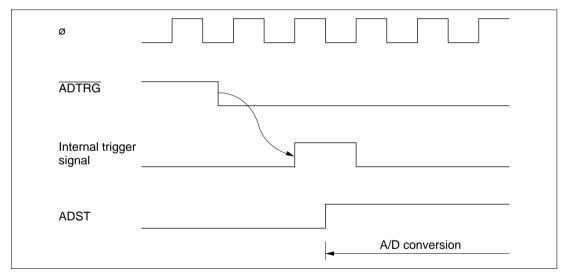
Figure 15.6 External Trigger Input Timing
