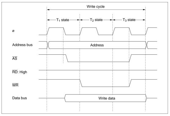
Figure 2.17 (b) External Device Access Timing (Write)
