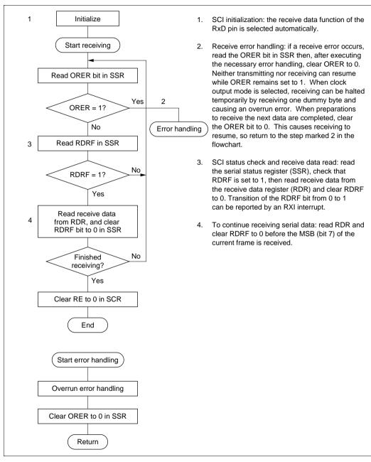
Figure 12.15 Sample Flowchart for Serial Receiving
