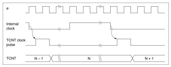
Figure 9.2 Increment Timing for Internal Clock Input
