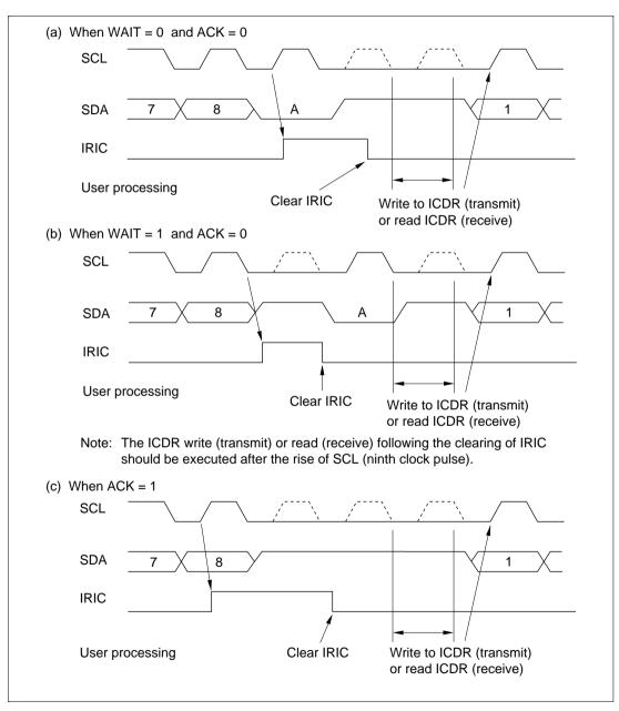
Figure 13.10 IRIC Set Timing and SCL Control
