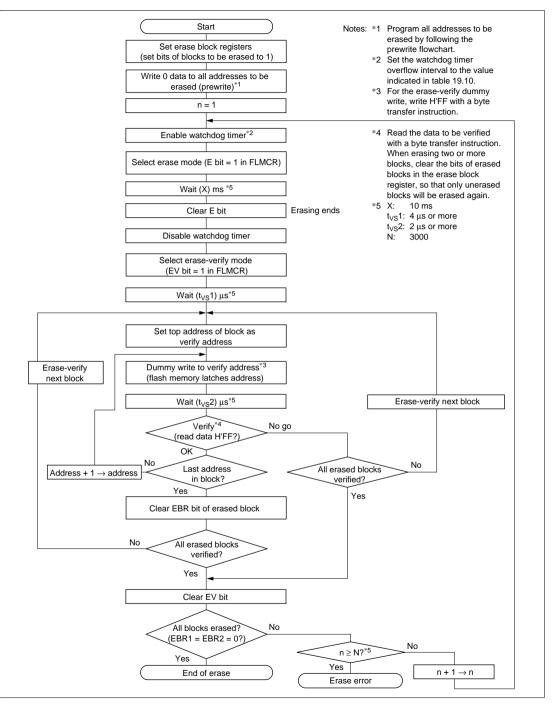
Figure 19.11 Multiple-Block Erase Flowchart
