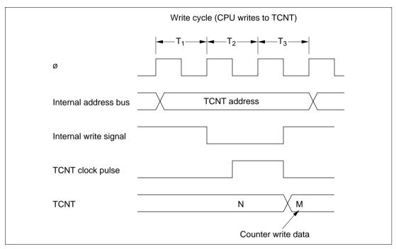
Figure 11.6 TCNT Write-Increment Contention
