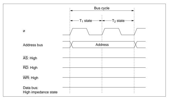
Figure 2.14 Pin States during On-Chip Memory Access Cycle
