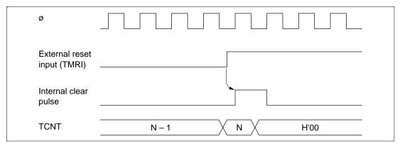
Figure 9.7 Timing of External Reset
