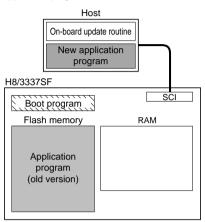
3. Flash memory initialization The erase program in the boot program area (in RAM) is executed, and the flash memory is initialized (to H'FF). In boot mode, total flash memory erasure is performed, without regard to blocks.
