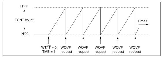
Figure 11.4 Operation in Interval Timer Mode
