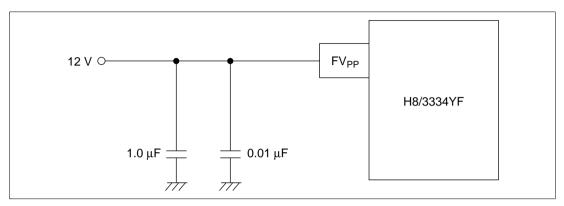
Figure 19.21 V<sub>PP</sub> Power Supply Circuit Design (Example)
