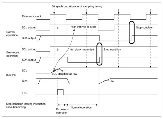
Figure 13.18 Stop Condition Erroneous Operation Timing
