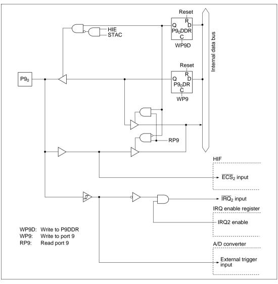
Figure C.9 (a) Port 9 Block Diagram (Pin P9<sub>0</sub>)
