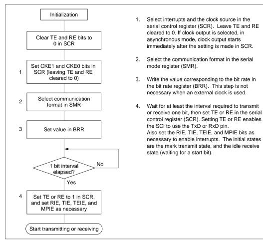
Figure 12.4 Sample Flowchart for SCI Initialization
