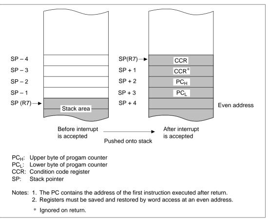
Figure 4.6 Usage of Stack in Interrupt Handling
