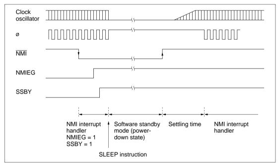
Figure 22.1 NMI Timing in Software Standby Mode (Application Example)
