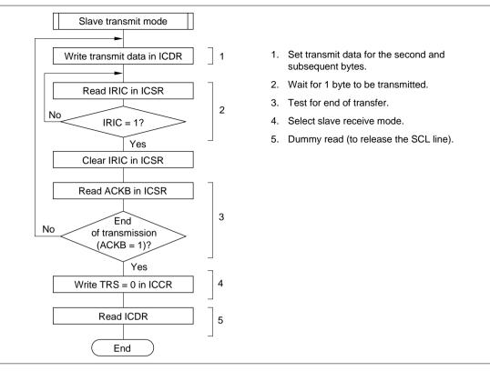
Figure 13.14 Flowchart for Slave Transmit Mode (Example)
