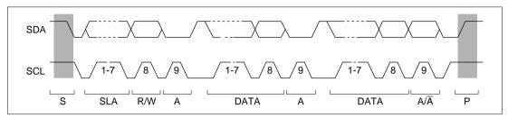
Figure 13.5 I<sup>2</sup>C Bus Timing
