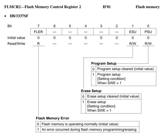
Note: The FLSHE bit in WSCR must be set to 1 in order for this register to be accessed.
